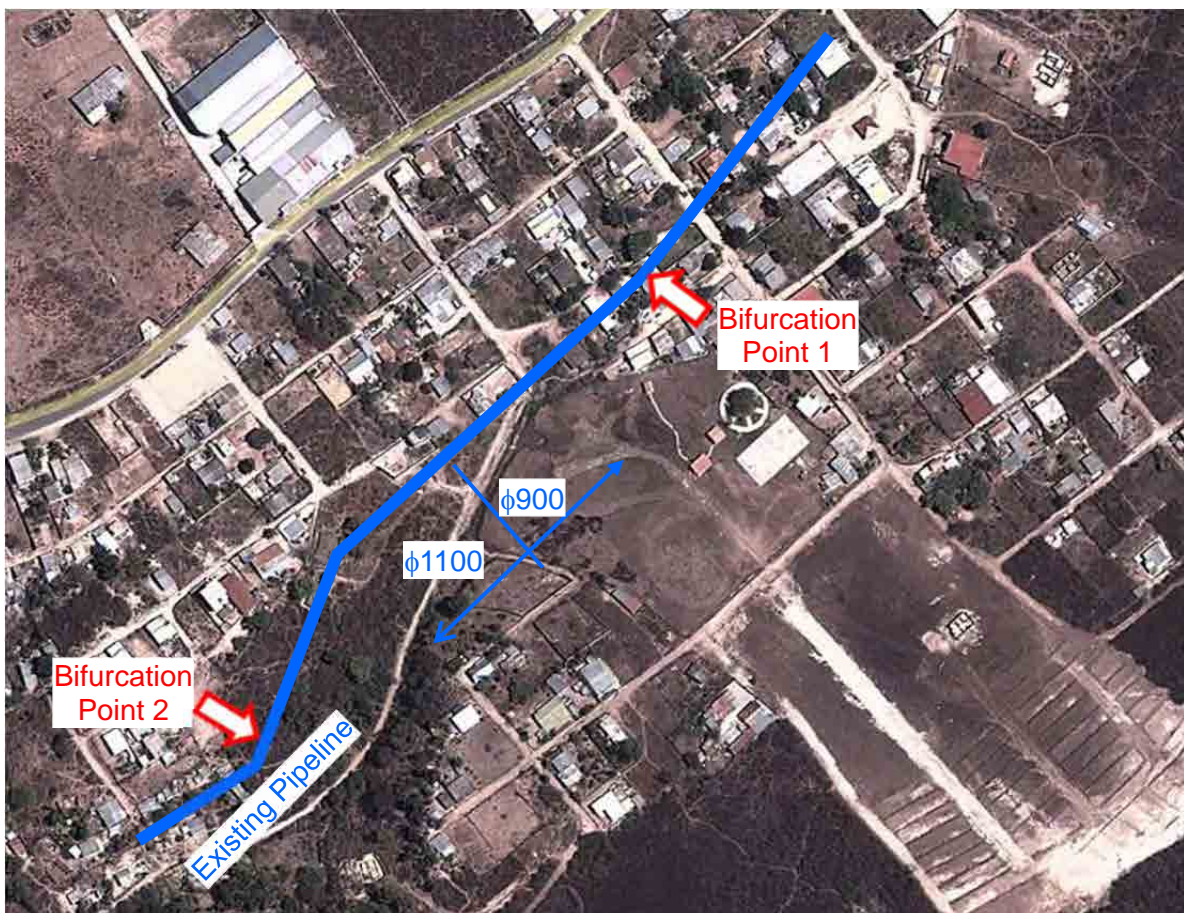
Fig. 2-2-21 Upstream Bifurcation Point of New Pipeline Route
