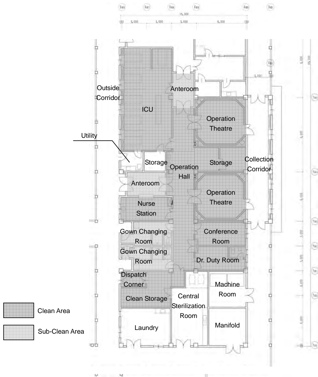
Fig. 2-5 Operation & Central Sterilization Dept. Plan Scale: 1/200
