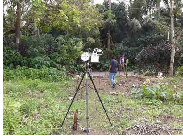
AQL2 Sulfur Dioxide (SO 2 ) and Nitrogen Dioxide (NO 2 ) level measurement at the residential area in along Silang-GMA Road in Brgy. Sabutan, Silang Cavite ( Sta. 2 ) on 22 December 2011.
