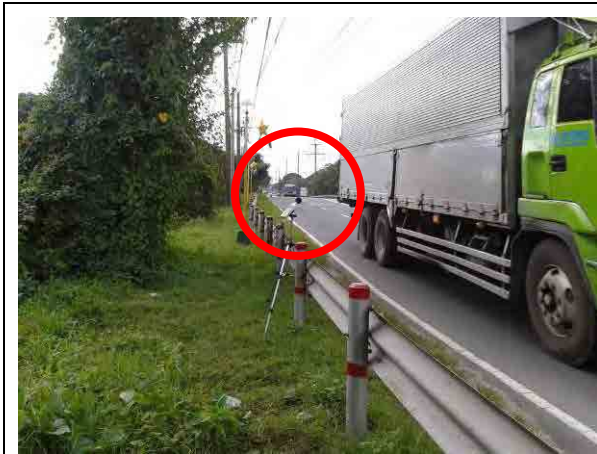
Sta. 1 Daytime noise level monitoring at sampling Sta. 1 .
