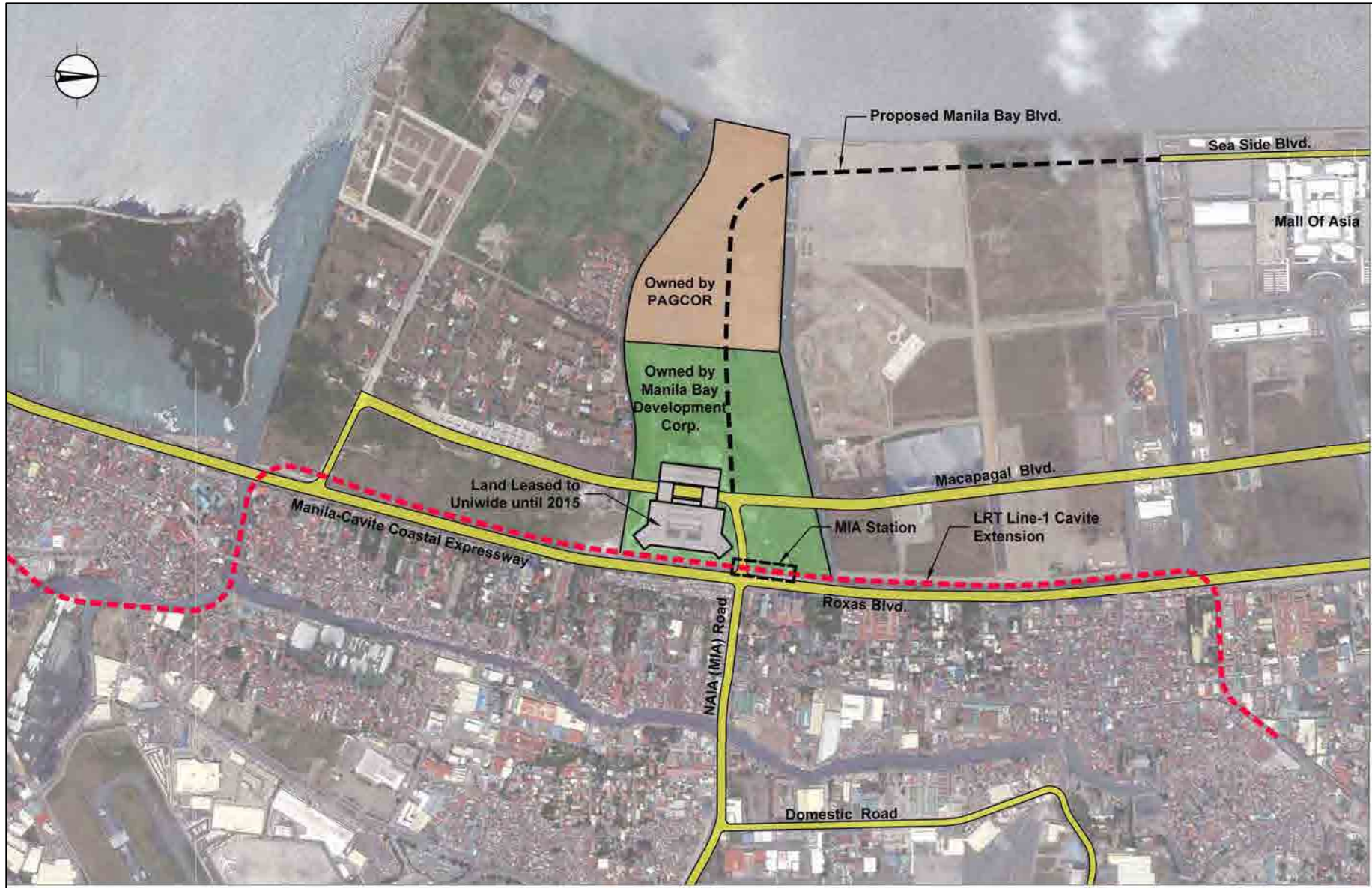
FIGURE 3.2.1-1 LRT LINE-1 CAVITE EXTENSION AND LAND OWNERSHIP
