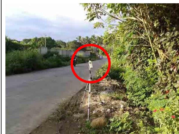
Sta. 3 Daytime noise level monitoring using a portable Noise Meter at sampling Sta. 3 , Brgy. Tibig, Silang, Cavite.
