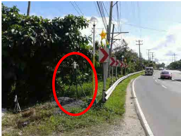
AQL1 Ambient TSP level sampling along E. Aguinaldo Highway, Brgy. Biga II, Silang, Cavite ( Sta. 1 ) using a Staplex High-Volume Sampler (indicated by the red marking).
