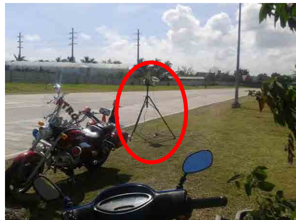
AQL4 Afternoon TSP level monitoring along the Nuvali-Laguna Boulevard, Brgy. Santo Domingo, Sta. Rosa City, Laguna, Sta. 4 .
