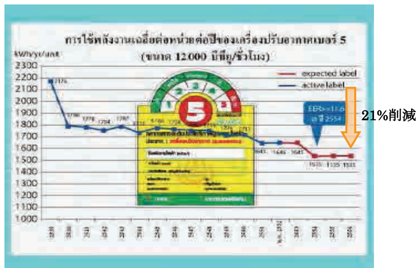
図 4.1.16 Resulting Energy Efficiency Improvement in Air Conditioners(12,000 BTU/Hr)
