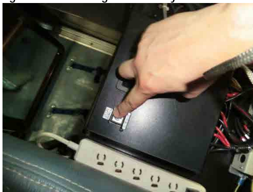
Figure 3.30 Shutting Down the System
