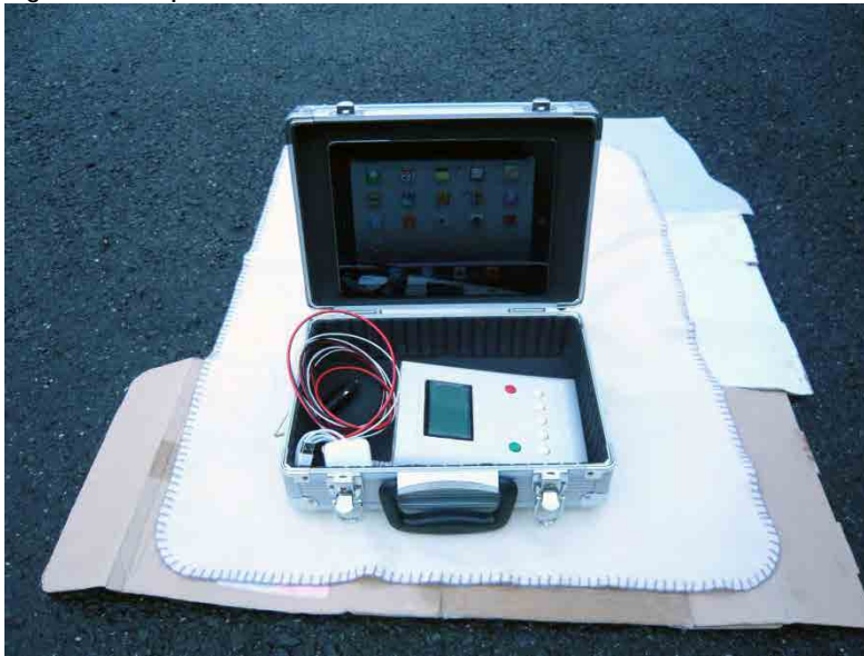
Figure 2.3 Trip Meter in an Aluminum Case
