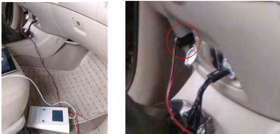
Figure 2.6 Power Cable Connection
