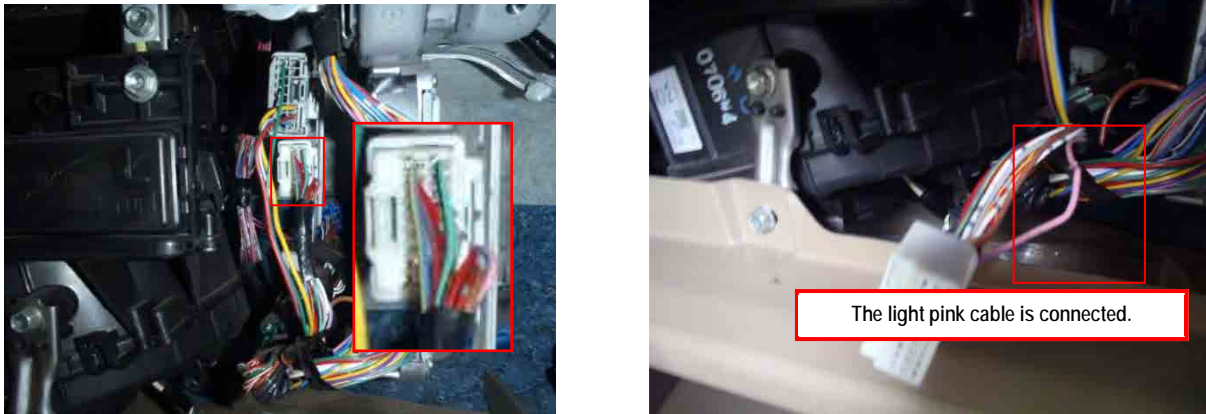
Figure 2.5 Vehicle Speed Pulse Signal Cable (Toyota INNOVA)
