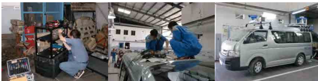
Figure 11 Setting Up Equipment to the Road condition survey vehicle
