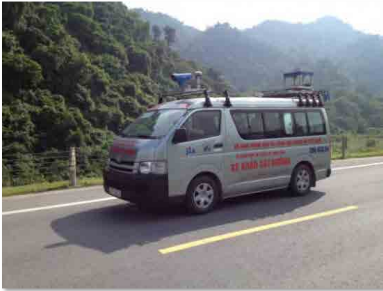
Figure 16 Pavement Condition Survey Vehicle in Operation
