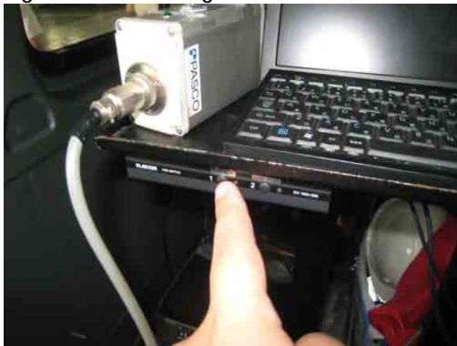
Figure 3.14 Switching PC1 and PC2
