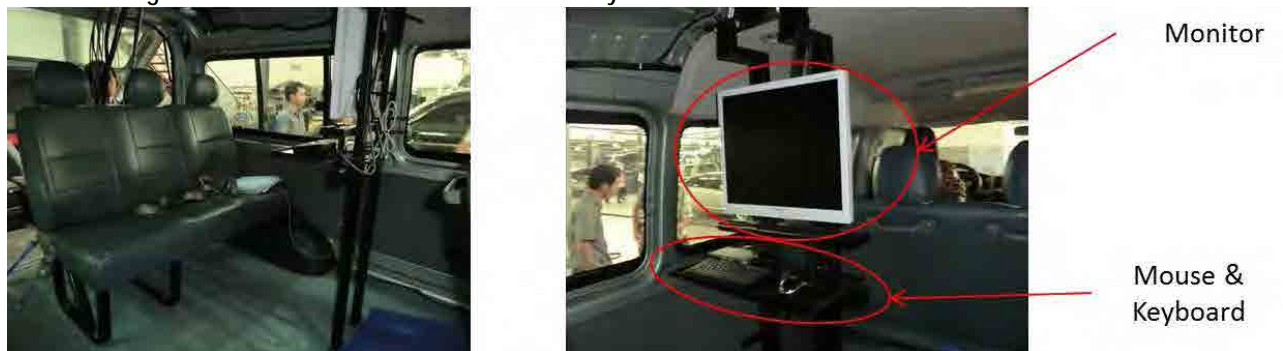
Figure 3.2 Inside of the Road Condition Survey Vehicle
