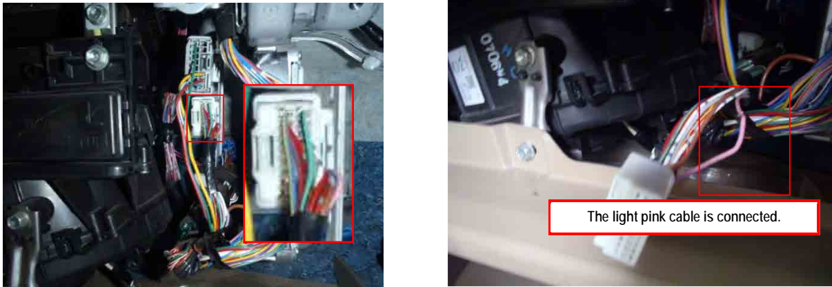
Figure 2.5 Vehicle Speed Pulse Signal Cable (Toyota INNOVA)
