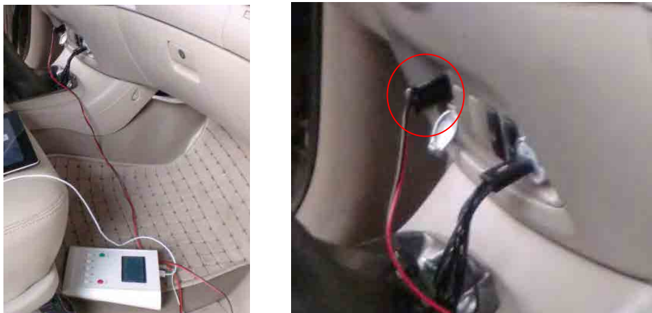
Figure 2.6 Power Cable Connection
