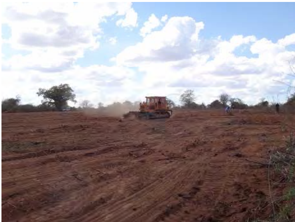
Removing bush trees by rake dozer
