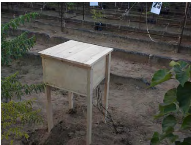
Photo 2. A box made of wood to store the water content meter and thermometer.
