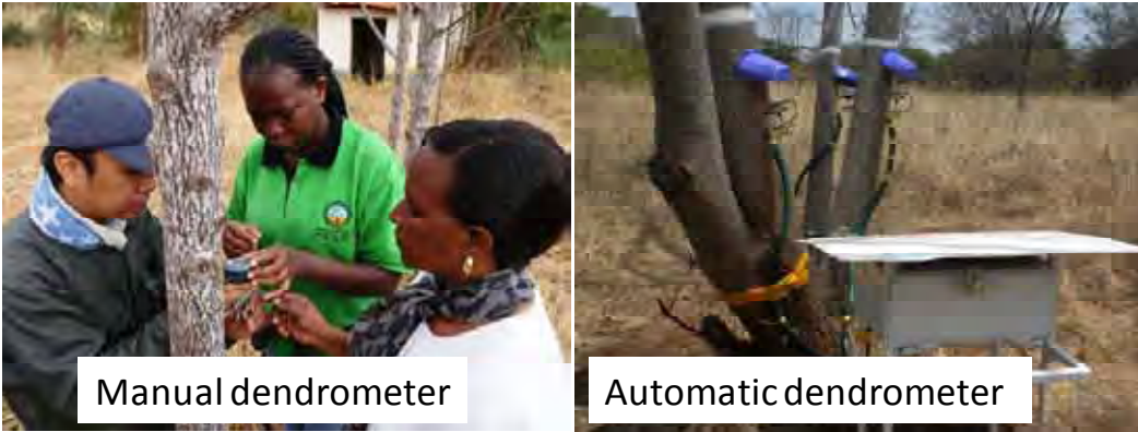
Fig.4 Installation of two types of dendrometer
