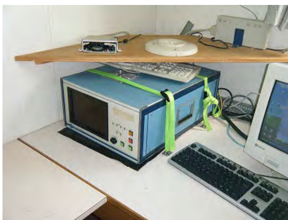
R/V “AMA” Acoustic Doppler Current Profiler
