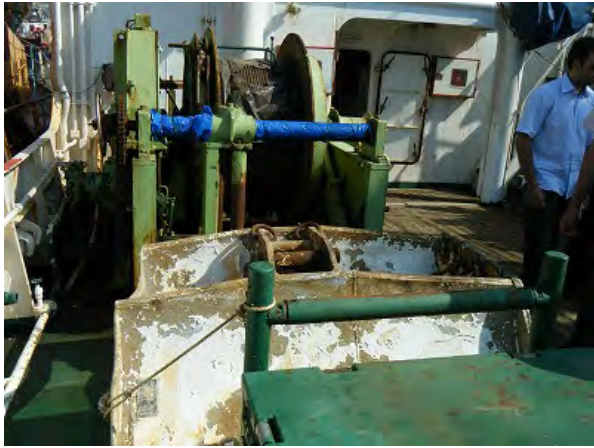
R/V "AMA" Port side Trawl Winch
