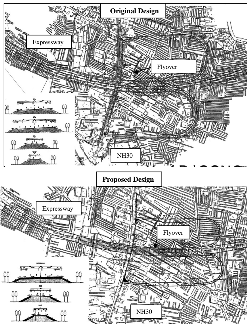
Figure 6.16. Original Design and Proposed Design of An Thai Trung IC
