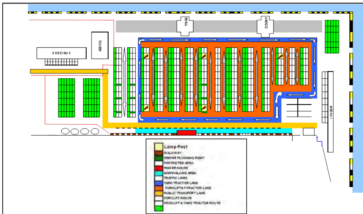
Figure 4-13 Yard layout of Suva Container Terminal
