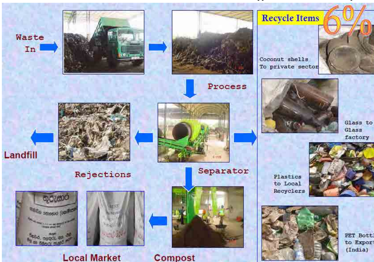
Figure 11: A process of compost production in Bloemendal site
