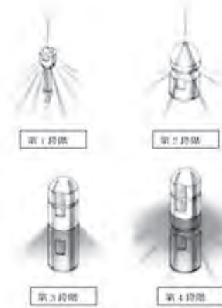
Figure 5.6.2 Flushing of Drainage Pipe
