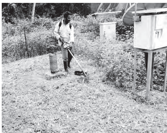
Photo 15 Cleaning of AWS Station
