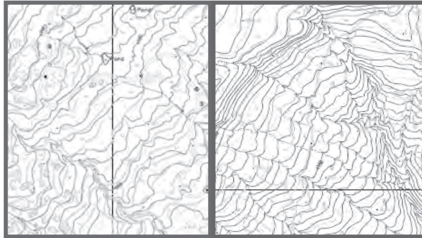
Figure 2.2.5 Comparison of Contour Lines on a Landslide Area (left) and an Area with no Landslides (right) *13
