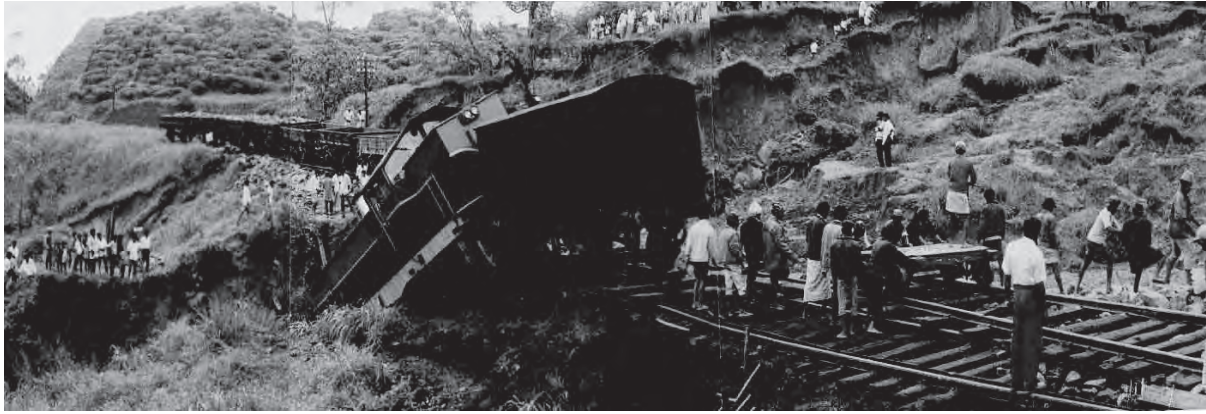
Figure 1.3.2 Damaged Train by the Watawala Landslide (NBRO)
