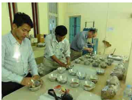
Preparation of Soil Specimen
