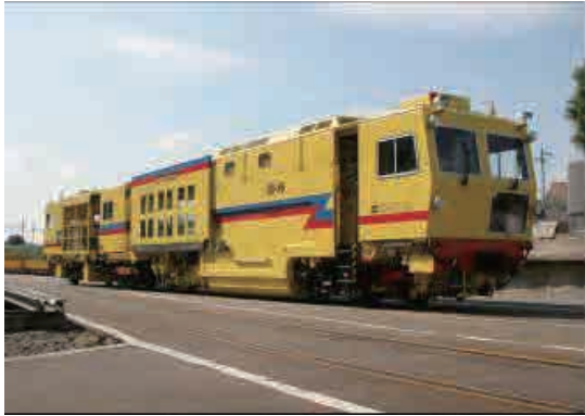
Source: JICA Study Team Figure 3.5.10 Tamping machine
