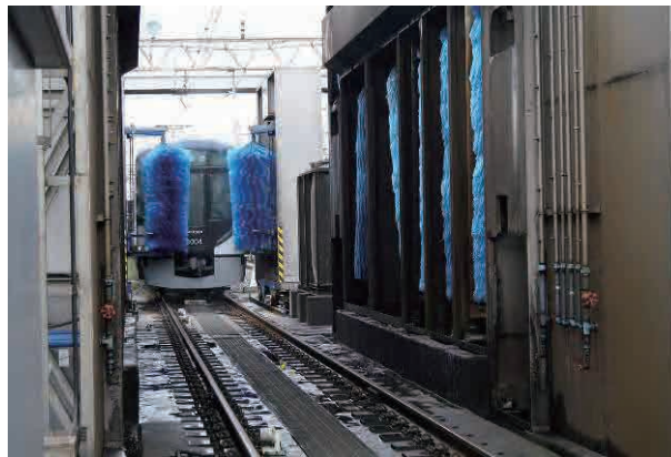
Source: JICA Study Team Figure 3.5.5 Car-washing track
