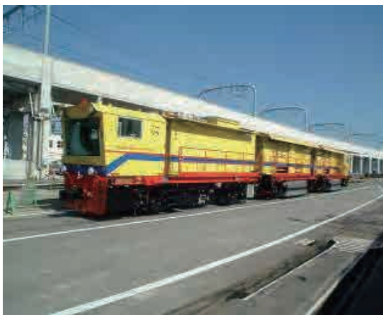
Source: JICA Study Team Figure 3.5.12 Rail grinding machine
