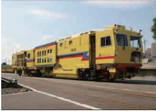
Source: JICA Study Team Figure 3.5.10 Tamping machine
