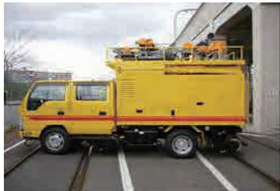
Source: JICA Study Team Figure 3.5.15 Overhead contact line inspection car
