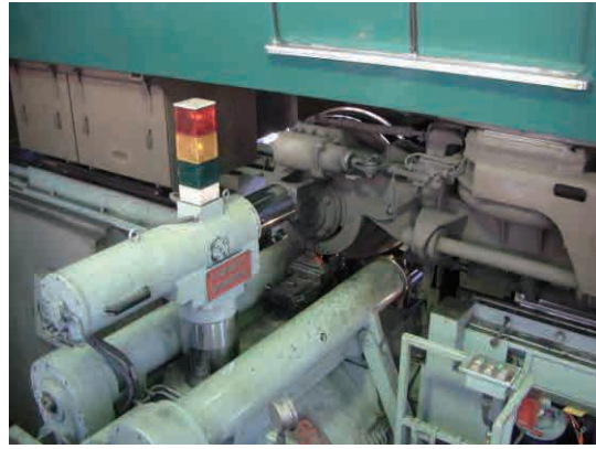
Source: JICA Study Team Figure 3.5.4 Under-floor type car wheel lathe (wheel lathe turning)
