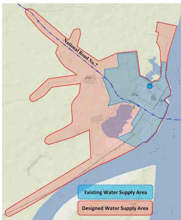
Figure 2.2.2.6-2 Designed water supply area (KMC)
