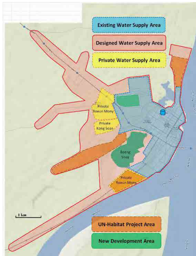
Figure 2.2.2.1-1 Future Water Supply Area in Kampong Cham
