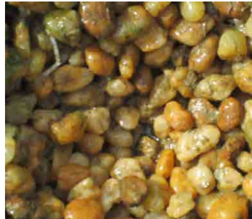
Roughing Filter : 5cm from surface
