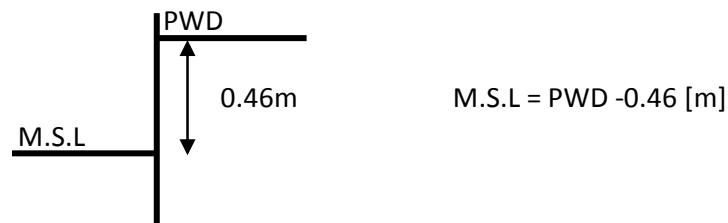
Figure 5.3.2 Relationship between BWDB's PWD.m and M.S.L.m
