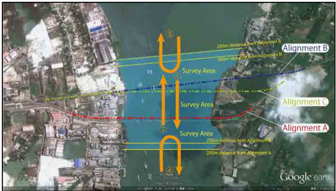
Figure 2.4.2 Survey Area (Meghna Bridge)
