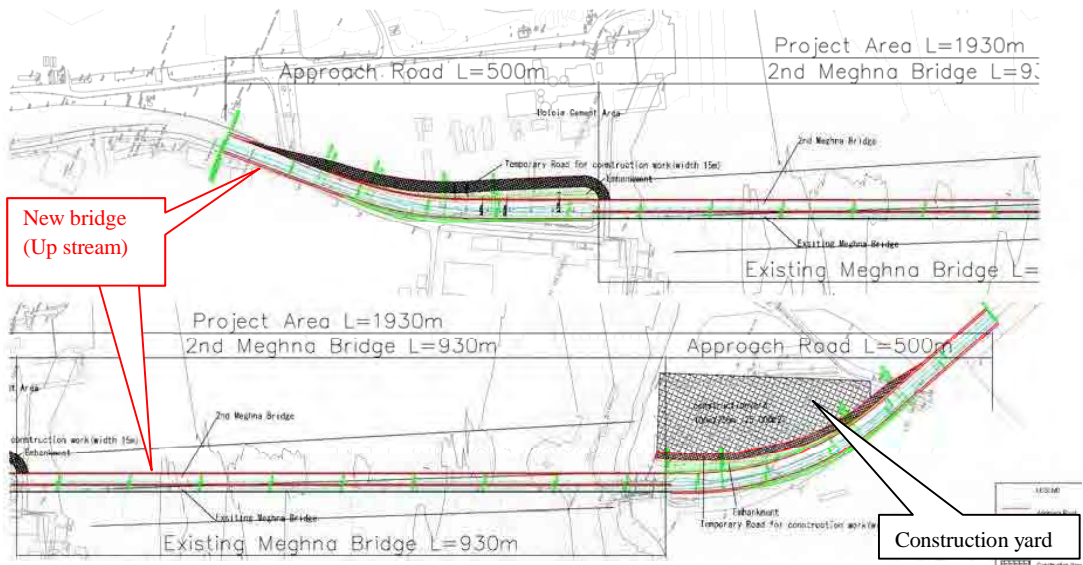
Figure 2.4 Locations of New and Existing Meghna Bridge with Construction Yards
