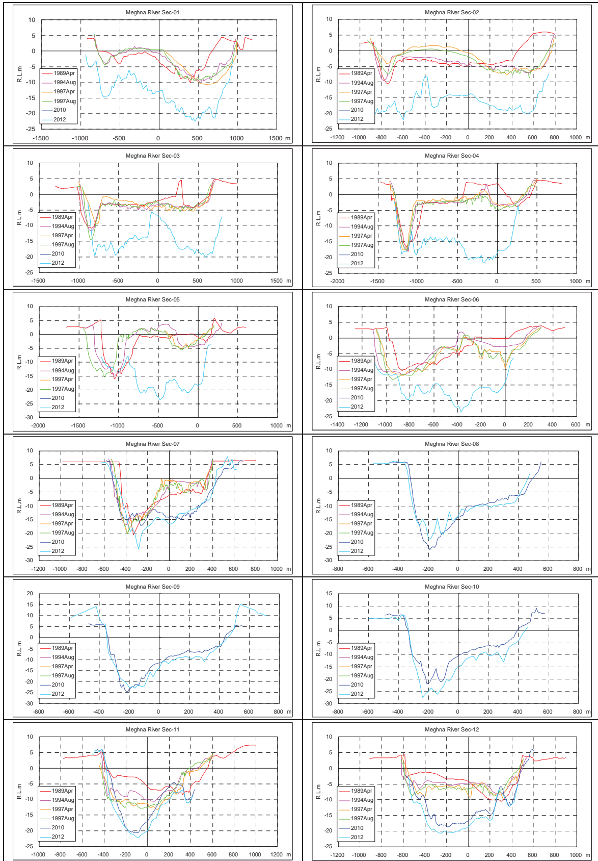
Figure 2.4.1 Historical Change of Cross Section Profile around Meghna Bridge
