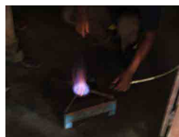
Biogas at burner
