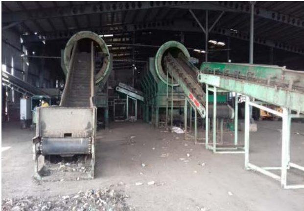
25mm screen machine in compost plant
