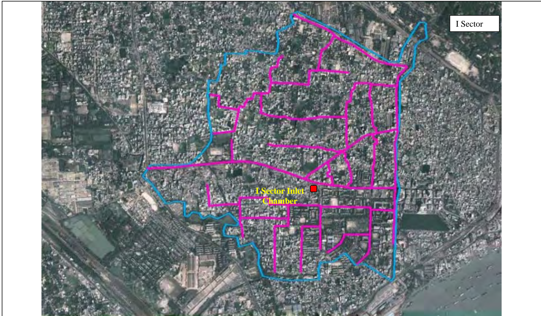
Figure 6.2.9 (9) Distribution Pipeline in Sector – I
