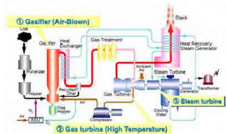
Figure 5.2-1 Integrated Coal Gasification Combined Cycle (IGCC)
