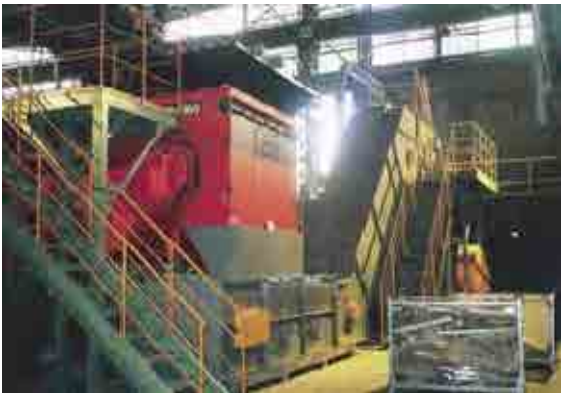
Image 5.1-5 Shredder for Used Plastics
