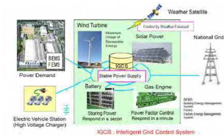
Figure 5.4-2 IGCS for a Factory Smart Grid (Hitachi)
