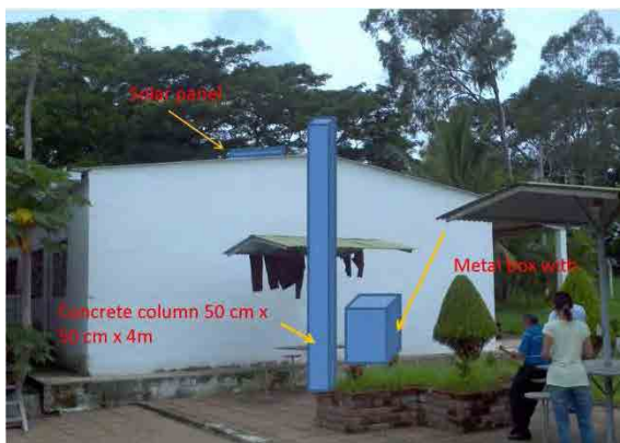
Install position of GPS sensor 2
