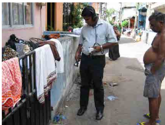
Kotahena Leak Detection (Acoustic Survey)
