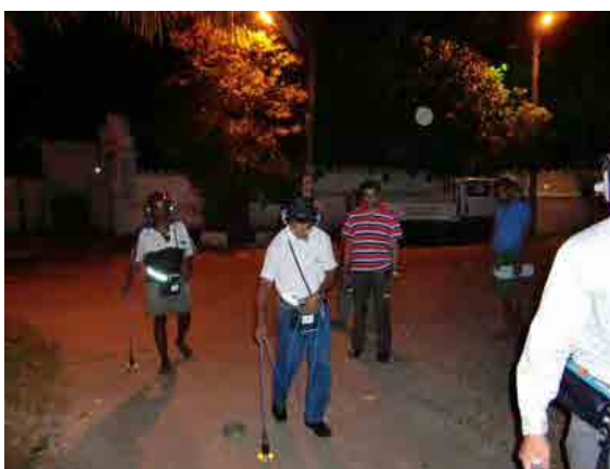
Borella Leak Detection (Pinpoint Survey)
