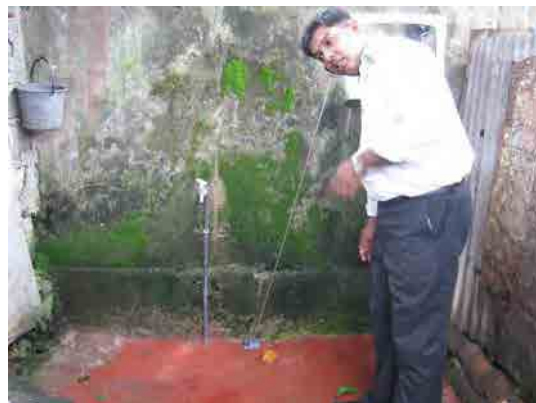
Kotahena Leak Detection (Acoustic Survey)
