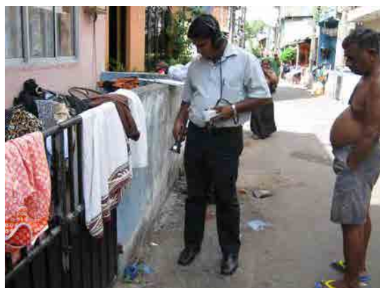
Kotahena 漏水調査 (Acoustic survey)
