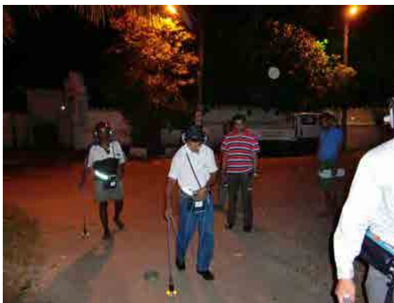
Borella 漏水調査 (Pinpoint survey)
