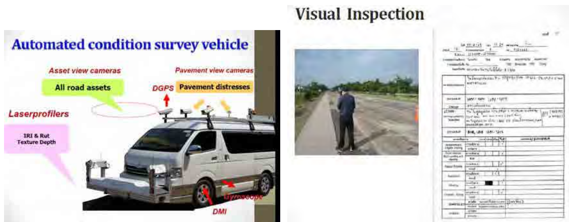
Fig. 4-6 Road surface property measurement vehicle and visual inspection (Thailand)
