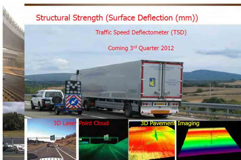
図 5-55 Structural Strength Survey Vehicle(SANRAL 資料)
