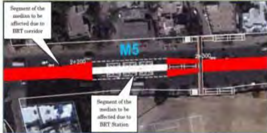
Figure 7.5: Example showing the affected segment of road when BRT is at median and location of stations
