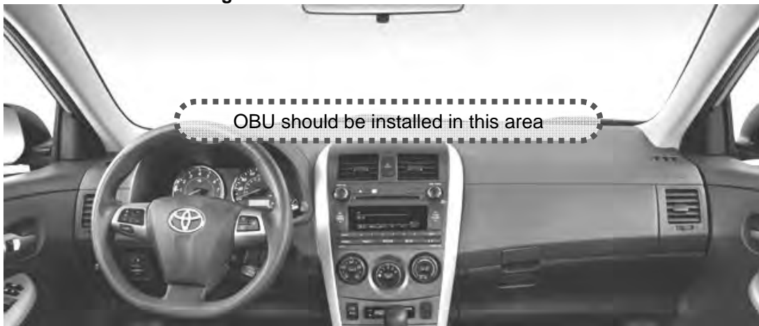
Figure 7.3 Installation of OBU in Vehicle
