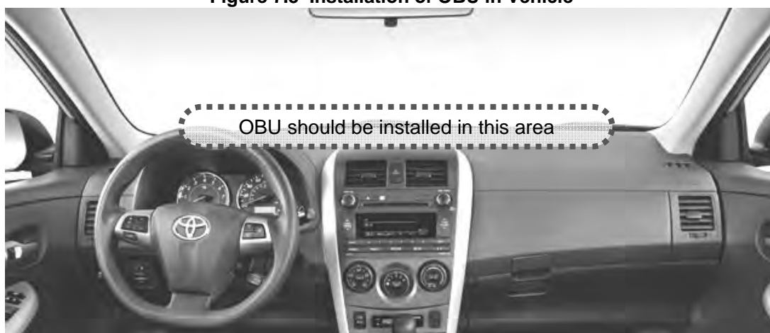
Figure 7.3 Installation of OBU in Vehicle
