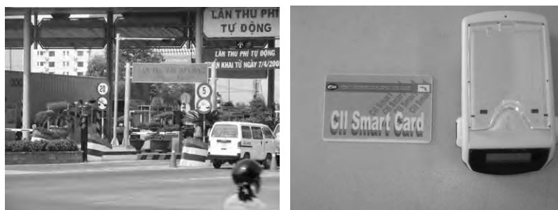
Figure 5.38 Tollgate Lanes and OBU with IC-card at Ha Noi Highway in HCMC
