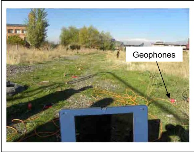
Figure 3.3-2 L-shape setting of geophones for surface wave exploration
