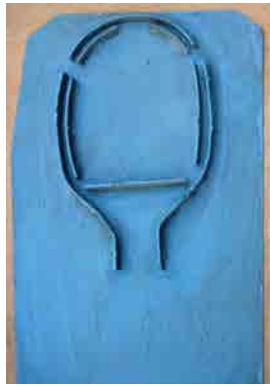
ANNEX 3 : Another type of mold for arranging the shape and welding work
