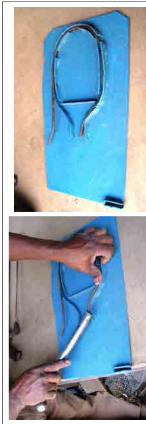
4 Bend the end part to arrange the shape. Push it into the mold.
