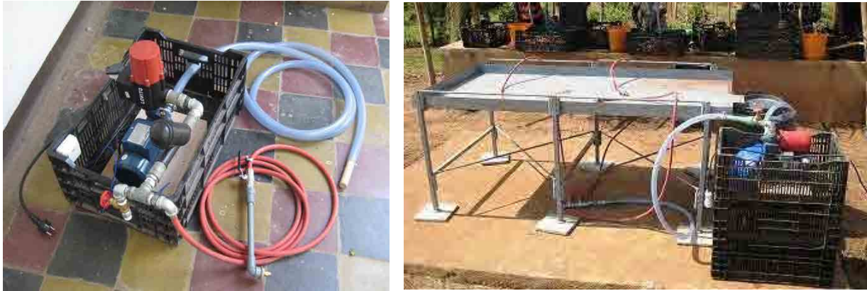
Device for final washing : “Jet-nozzle + constant pressure water” plus “water recycle system”
