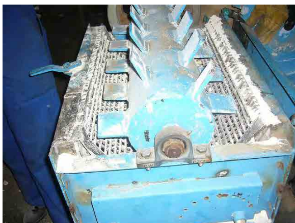
Drum type crusher was developed after repeated performance tests.
