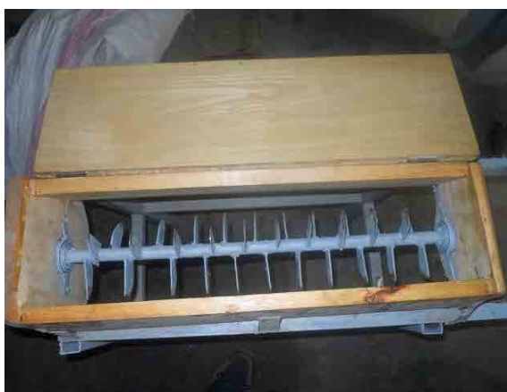
Hawassa University developed fiber cutter with multi knives for Kocho.
