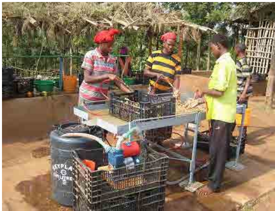
Final washing with Nozzles + Water pump
