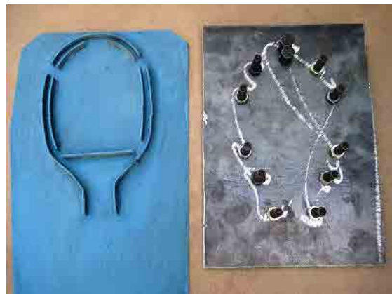
Left : Mold for bending/shaping and welding. Right : Mold for bending/shaping
