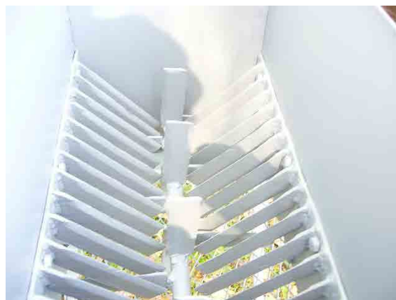
The installation angle of fixed blades is 45 degree for smooth discharge. The gap between the screen and edge of knives needs to be 5mm.
