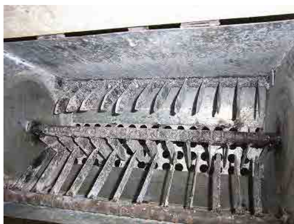
The Study team modified original Kocho cutter to fresh cassava cutter by installing fixed and rotating blades.
