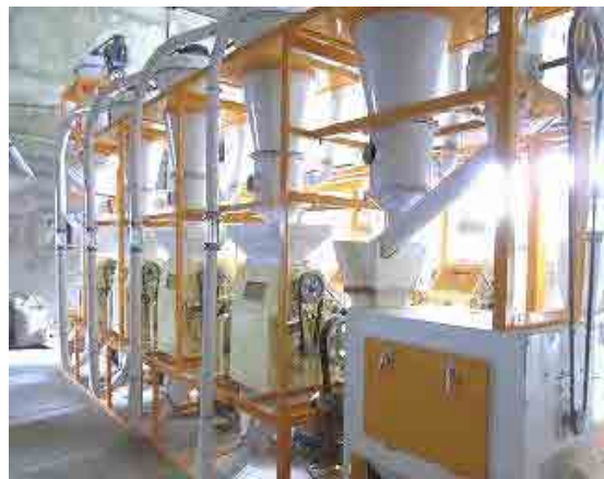
Roller mills unit
