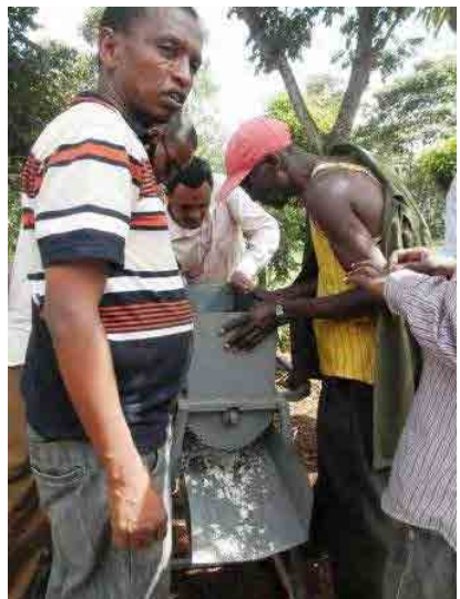
A participant tries to cut the cassava with the new cassava cutter developed by SAMS (PP04)
