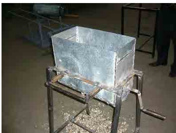
Proto type Cassava Cutter fabricated after many performance tests, sent for tests and monitoring by farmers in April.
