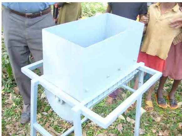
Improved model of cassava cutter. The body shape is circular for easy cutting and discharging.
