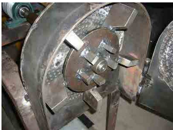
Pin Mill type dry cassava crusher.
