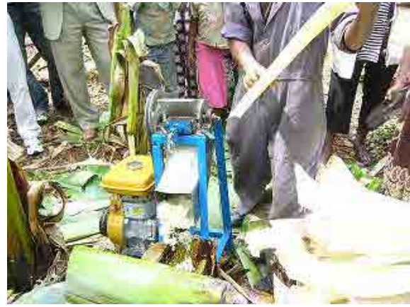
Drum type peeling machine driven by an engine. Drum cannot control peeling off the edible portion only, but with outer fibers.
