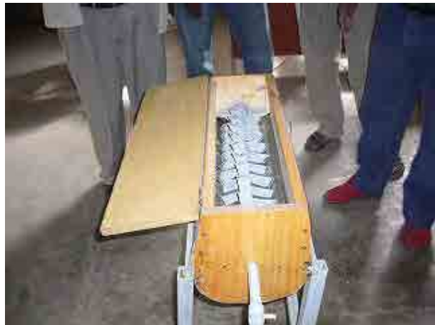
Hawassa University has developed multi-knives rotating cutter for Kocho fibers but is not finalized yet.
