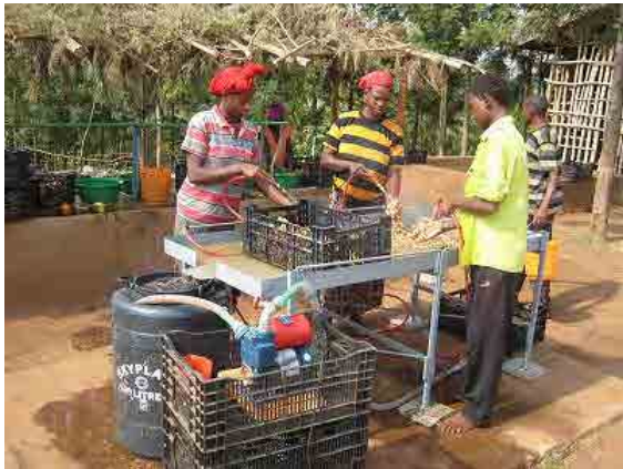
Final washing with Nozzles
