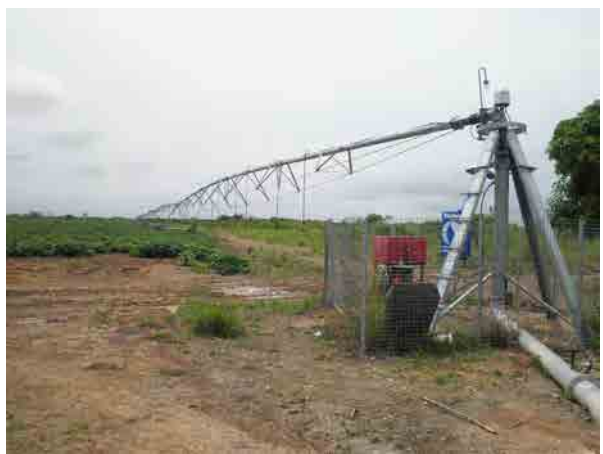
Center pivot system Cassi Farm applied center pivot sprinkler. Pumped up water is supplied from Volta river in 2km away from the farm. Photo shows soybean cultivation.
