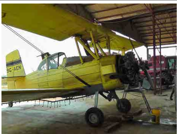
Prairie Volta Farm Air plane is used for seeding and pesticide spraying.
