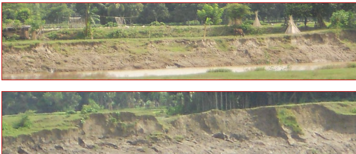
Image 3 Typical bank profile in proposed bridge site at Gudaria River ghat showing (L) sandy clay soil type, and (R) evidence of stiff clay soil near proposed bridge location
