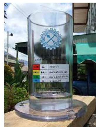
Figure 4.4.3 Simple Rain Gauge
