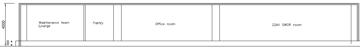
Fig. 3-3-7-3 Layout Image for Switchgear House
